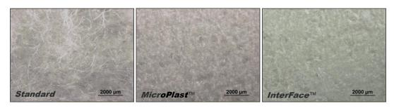
By its specific needling and finishing, InterFace™ calibrated surface reaches pressure uniformity and surface capillarity impossible to reach with traditional technologies, resulting in a consistent rewetting reduction.
