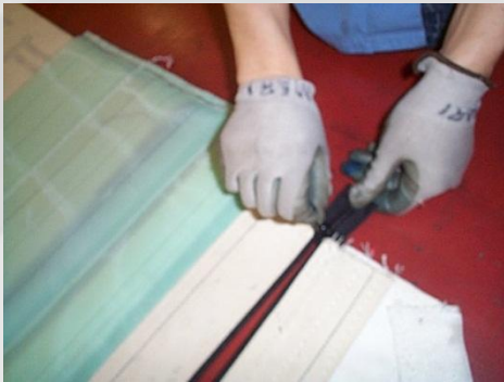
Locking of the leader to the felt
